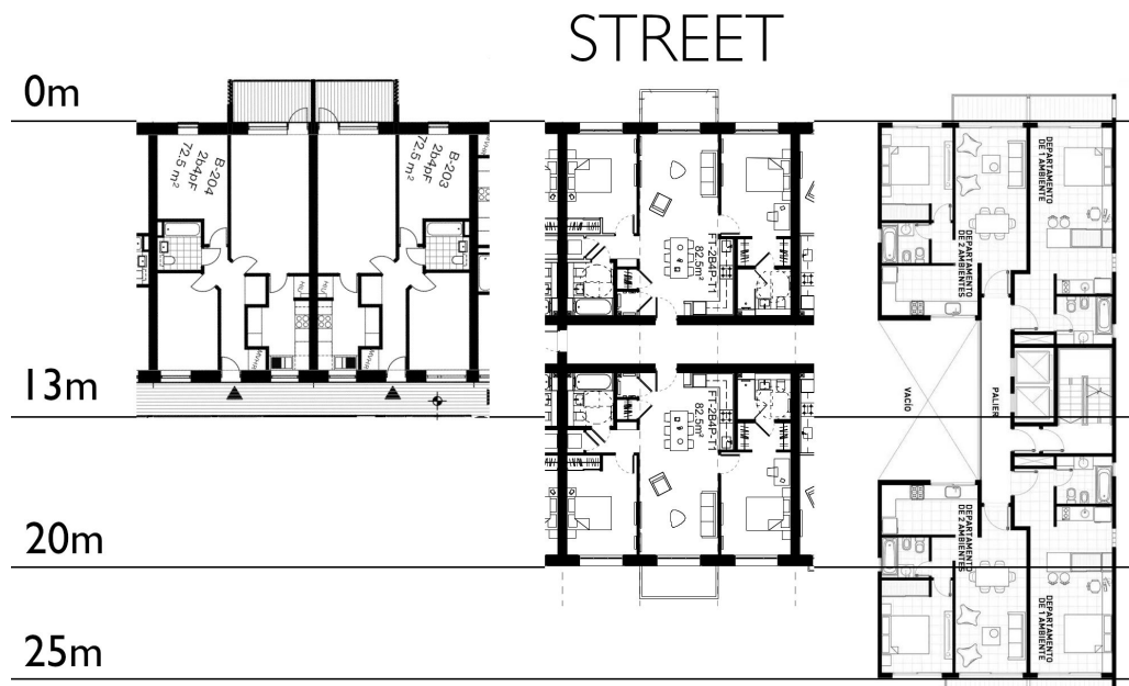
Figure 33: Building Typology and Plan Depth. Dual-aspect deck-access flats (London); single-aspect corridor-access flats (London); flats with light-well and lift-access (Buenos Aires)
